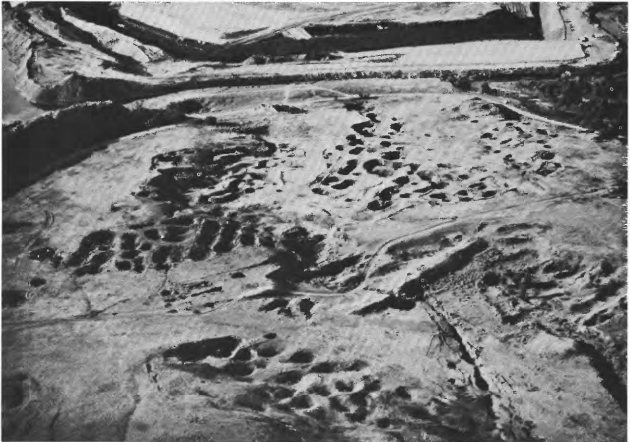
FIGURE 6.—Southeastward-looking aerial view showing the surface effects of past (room-and-pillar) and present (open pit) coal mining along the Tongue River in Wyoming (July 1977). Pits, troughs, depressions, and cracks have formed because of subsidence over the south part of the Acme mine. The mine was operated from the early 1900's until 1943. Overburden thickness ranges from 15 m in the middle ground to approximately 30 m in the foreground and consists of alluvium and soft interbedded shales, claystones, siltstones, and discontinuous sandstones. The dam in the right foreground across Hidden Water Creek ruptured because of subsidence. The water now is diverted into subsidence depressions, pits, and cracks upstream from the dam. Garbage from the town of Acme was dumped into the large pit at the left side of the photograph. Pits and troughs in the middle of the photograph are in alluvium. Note that the pits near the road and left of the draw do not occur in any noticeable depression; these pits are located above collapsed areas in haulageways of the Acme mine where adjacent coal pillars are strong enough to support the overburden. Alluvium is being removed at the Big Horn surface coal mine to extract the coal (background). Regrading is beginning near the river (right background). (From Dunrud and Osterwald, 1980.)
